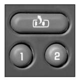
If your vehicle has this feature, then the controls for the memory function are located on the driver's door.
